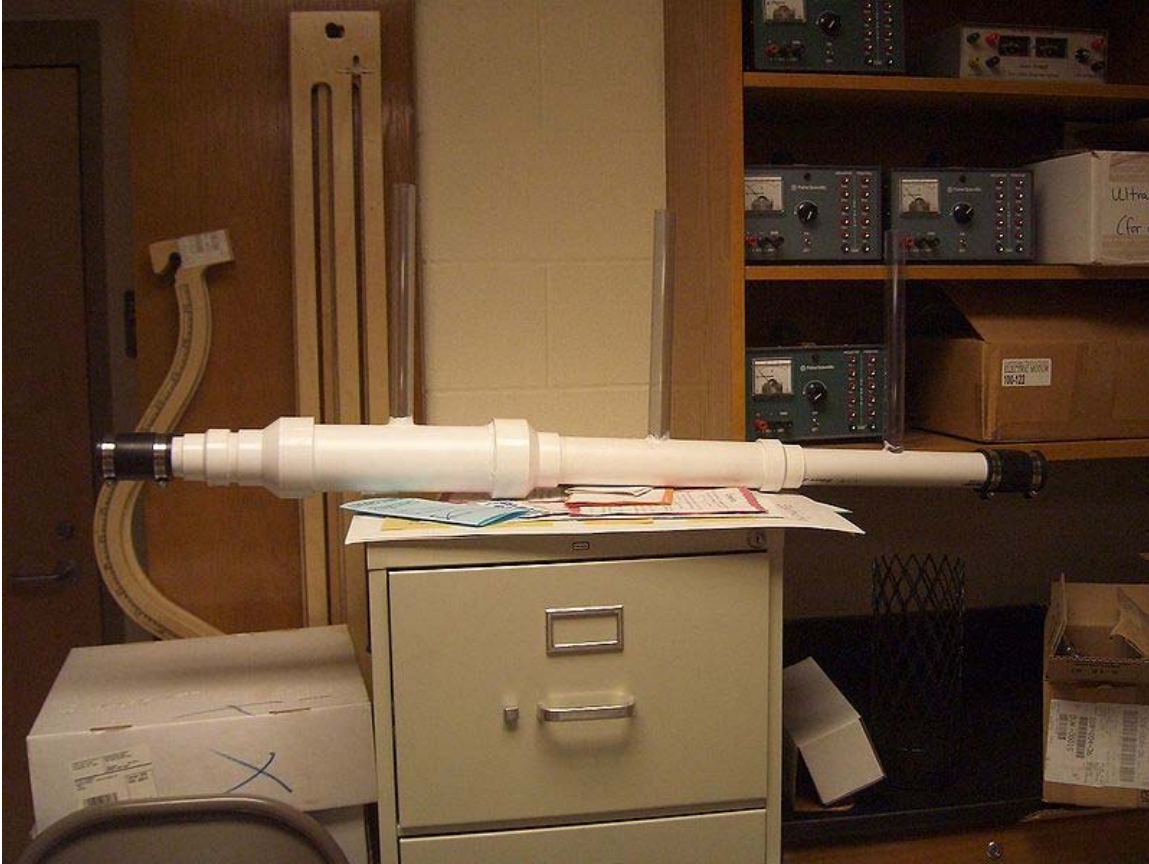
Venturi tube demonstration apparatus built out of PVC pipe and operated with a vacuum pump
